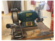
Ken brought along a Record Power grinder, which he had adapted by replacing the left hand wheel with a Cubic Boron Nitride (CBN) wheel, which can grind with less heat than a standard wheel (he got this from T&J Tools in Rugby).
