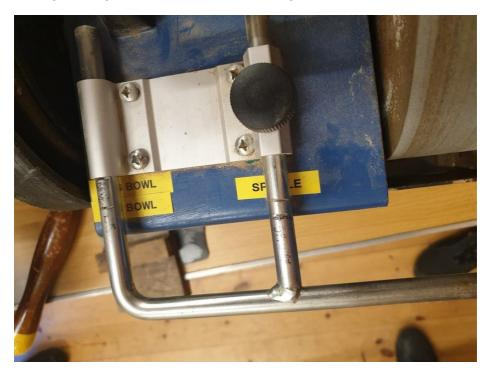
Roy has adapted his Tormek by marking the tool rest rods so that he gets the right distance from the wheel for different angles of grind for differing types of chisel.
